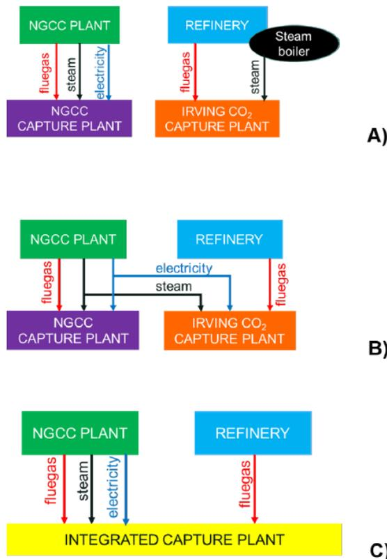
**Figure 5 Schematic layout of the three scenarios**
