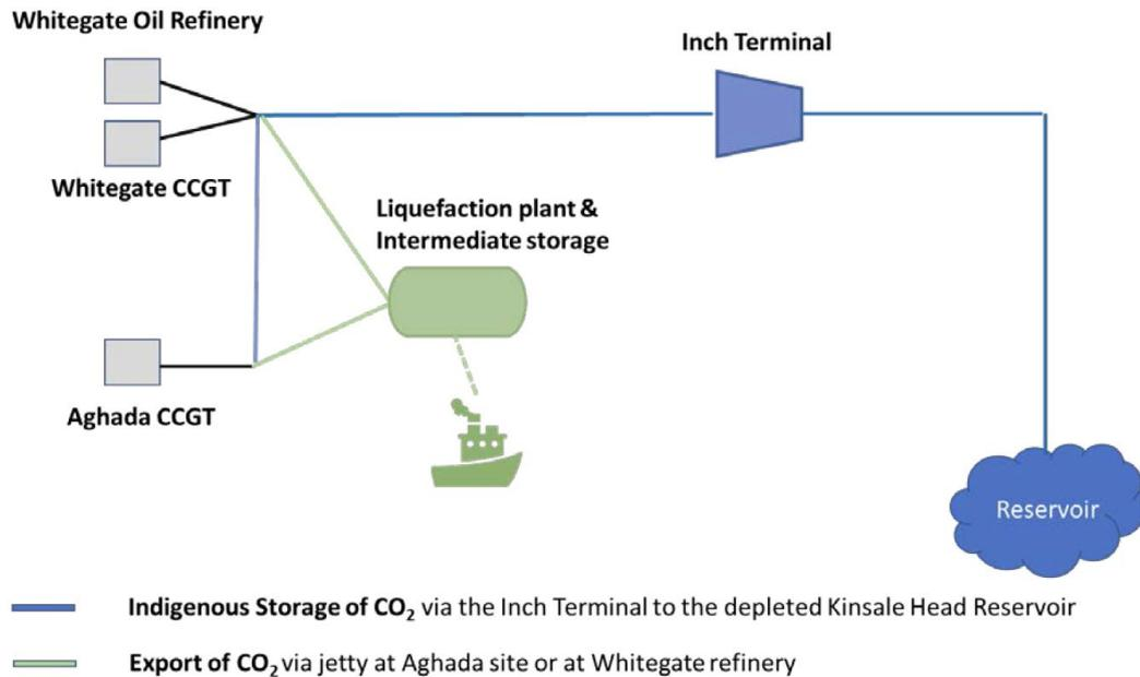
**Figure 4 Schematic layout of the system**
