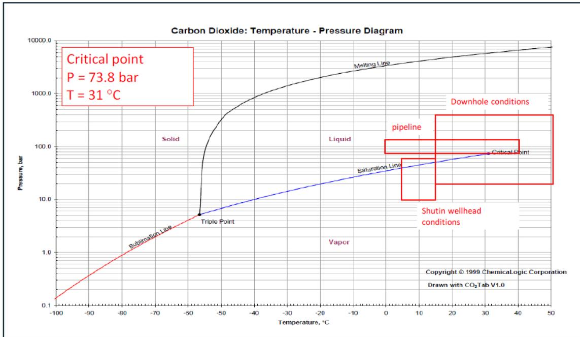
**Figure 3 Typical conditions in pipeline and injection well, for pure CO<sub>2</sub> transported in liquid phase**
